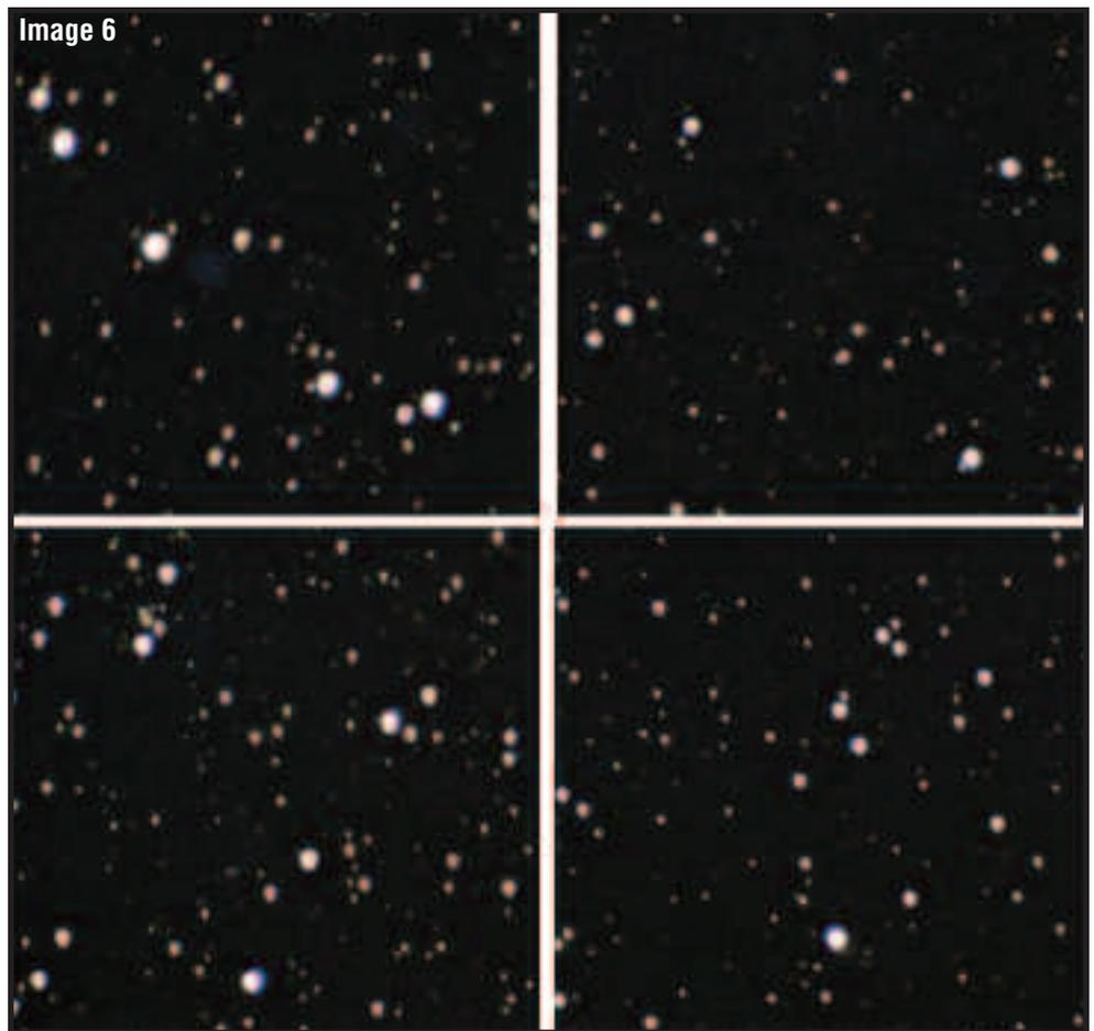
**Crops of the four corners of the same shot of M45 showing performance at the edges of an APS-sized frame (27 mm diagonal). Stars are sharp and round with no obvious aberrations.**
