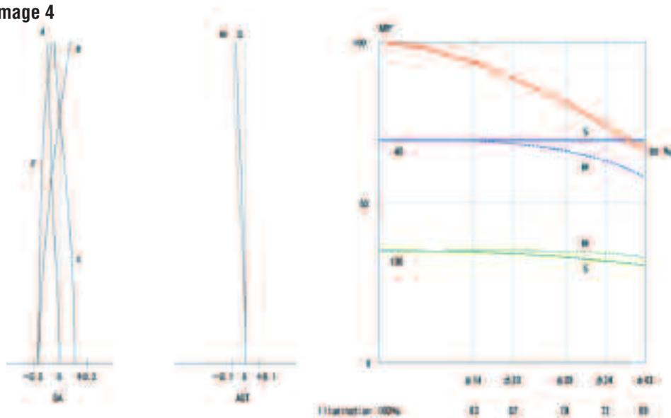
**Spherical aberration (left), astigmatism (middle) and combined percent-illumination and MTF data for the Borg 101 f/4. Diagram colored and used with permission from Hutech.**
