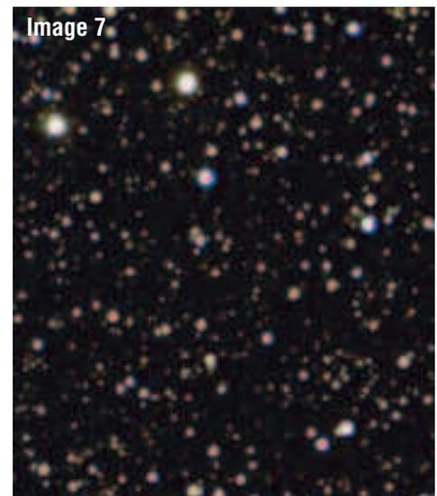
**(Corner\_Slight\_Defocus) Crop of a corner of a shot of the Rosette Nebula taken with a slight defocus. While stars are softer than optimal and careful inspection can show the defocus, there are no other readily apparent aberrations.**
