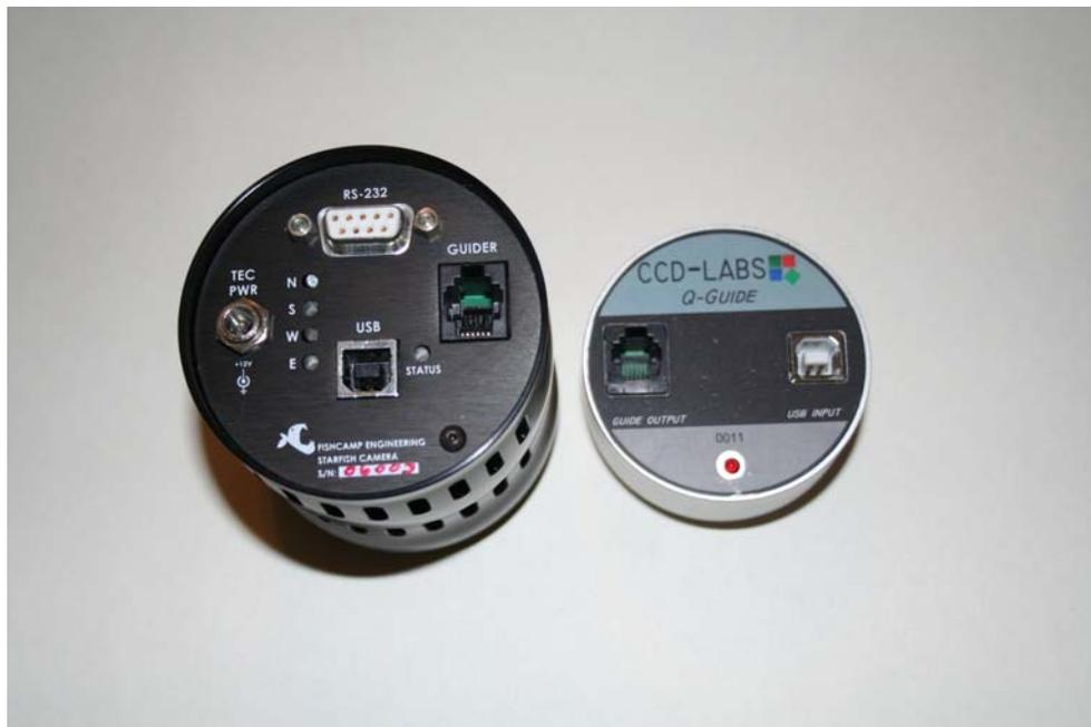
The port connections on that back of the Starfish (left) and Q-Guide.
