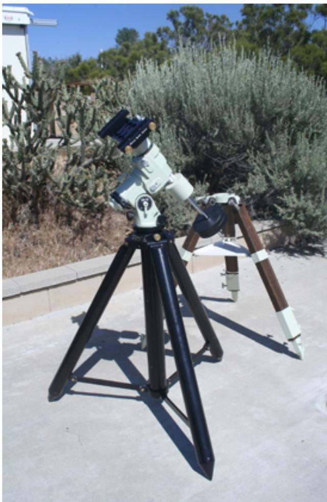
The tripods are not lightweight devices one might consider taking on a backpacking trip. The short version clocks in at 33 lbs, the tall and adjustable at 47 lbs. That said, for the level of stability they offer (they are rated to carry a 400 lb payload), they're quite portable.
